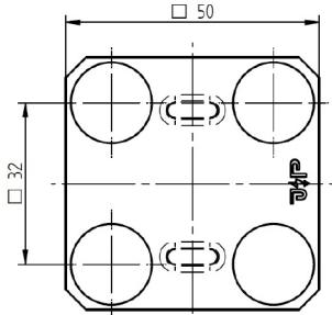
Copper cross clamp for flat conductors for use in T-, cross and parallel connections
